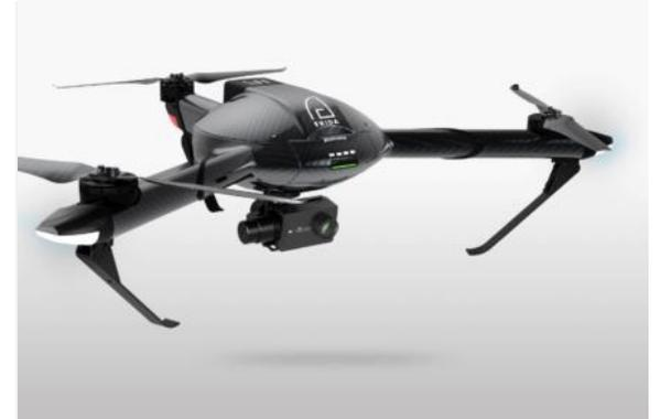
[YI's Erida](#) drone tricopter was developed with Atlas Dynamics. Made of light-yet-strong carbon fiber, YI says the tricopter can reach speeds of up to 75 mph (120 kph) and stay in the air for up to 40 minutes. A technology that could have an impact on e-commerce delivery solutions.
